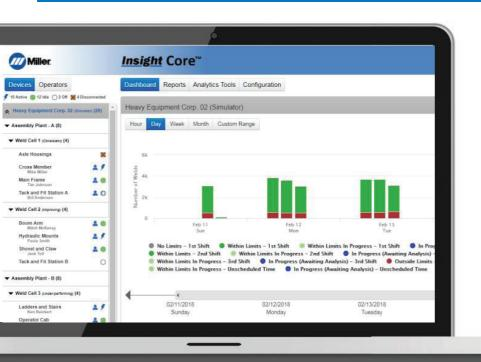
Do you know whether your company's welds are within acceptable ranges for amperage, voltage and wire-feed speed? Insight Core can tell you. It can also provide a date and time stamp, including a weld trace, for every weld. You'll have the necessary documentation to identify machines or welders that operate outside of expected parameters — so you can drive continuous improvement of the products you manufacture.
