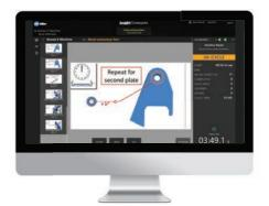
Insight Centerpoint guides the welder through the fabrication process from pre-weld to postweld in a standardized sequence.
